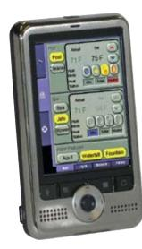
**iTC25 Kit (P/N 520501):** includes Wireless Personal Digital Assistant (PDA) with color touch screen custom-configured for IntelliTouch systems, wireless router and a Protocol Interface Adapter.
